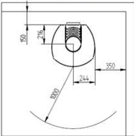
Distance to combustible WITH insulated flue
