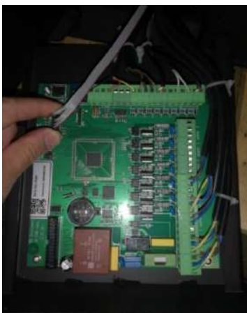
Picture 1: Unplug the display cable
