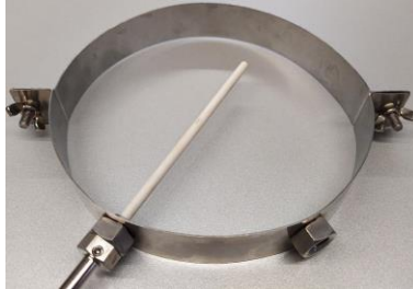
Pipe clamp with temperature sensor mounted
